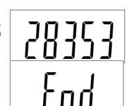
As soon as the weight, that is required for the calibration, will be indicated shortly at the display, the adequate calibration weight is to hang onto the scale. Then you have to wait until the value is stabilized.
